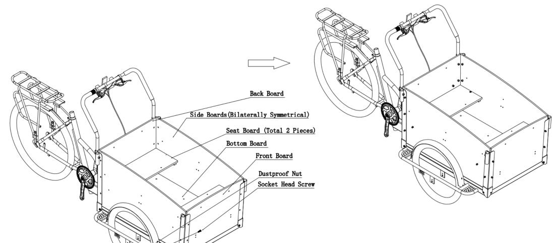
4. Put the front, rear, left, right wooden case boards inside the wooden case supports. Put the baseboard onto the chassis and fix the fastening screws. Fix the screws to connect the front, rear, left, right wooden case boards with wooden case supports. Put the two seat boards in place and fix with fastening screws.
