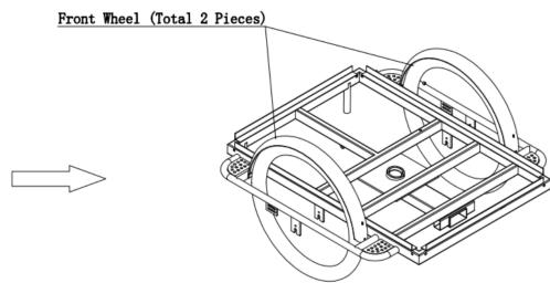
1. Fix the fender on the fender support of the chassis. Install the two front wheels onto the chassis. The deviation of the front wheels to the left and right sides shall be controlled within ±1mm. Fix the fastening screws in place. The two front wheels shall rotate flexibly. Fix the Rolla brakes with fastening screws.
