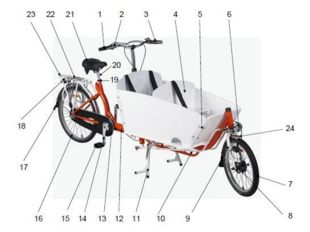
1.Handle bar & brake lever 2.gear shift 3.brake lever 4.box 5.comer iron 6.front light
